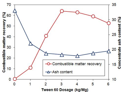
Fig. 2. Flotation results at different Tween 60 dosages
