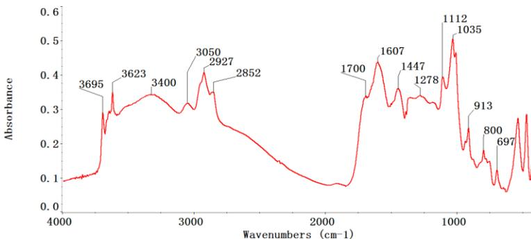
Fig. 1. FTIR spectrum of long flame coal
