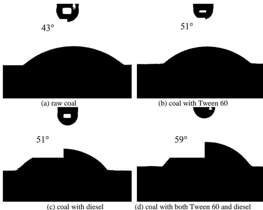
Fig. 5. Static contact angles of different coal tablets
