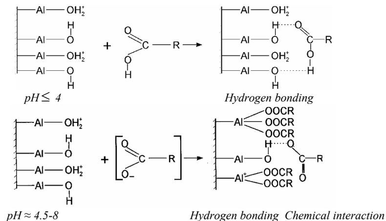
Fig. 3. PAA macromolecule - Al<sub>2</sub>O<sub>3</sub> surface interaction (Santhiya et al., 19990)
