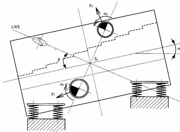
Fig. 19. Linear-elliptic screen with a stepped sieve
