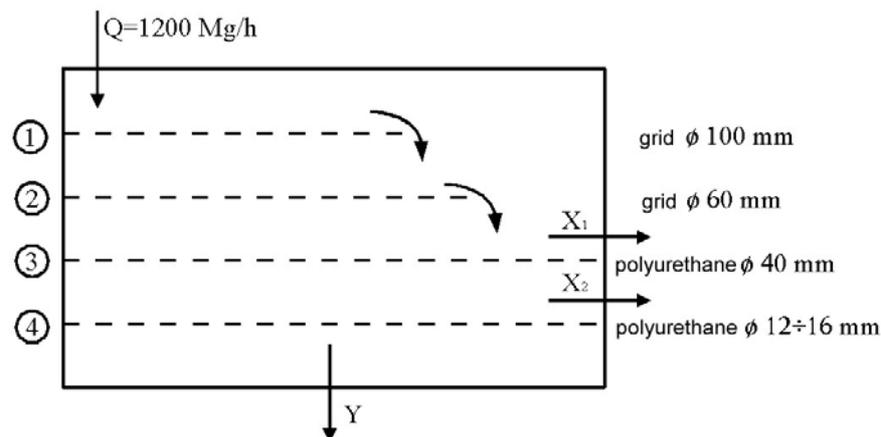
Fig. 2. Schematic of crude ore screening
