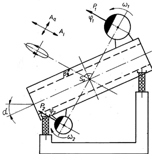
Fig. 9. Inclined linear-elliptic screen
