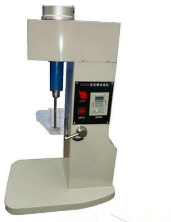
Fig. 2. View of XFG laboratory flotation cell
