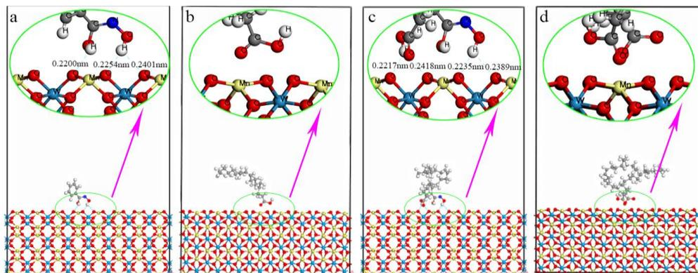
Fig. 7. Equilibrium adsorption configurations of a – HA, b – HOL, c – mixed HA–HOL, d – mixed OL<sup>–</sup>–HOL on the huebnerite surfaces obtained by molecular dynamic simulations
