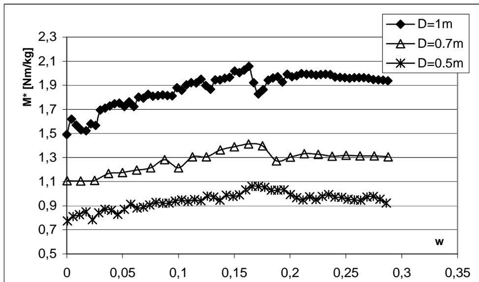
Fig. 5. Example of changes in reduced torque with bed moisture content for three disk diameters ( $k=7\%$ ,  $\alpha=45^\circ$ )
