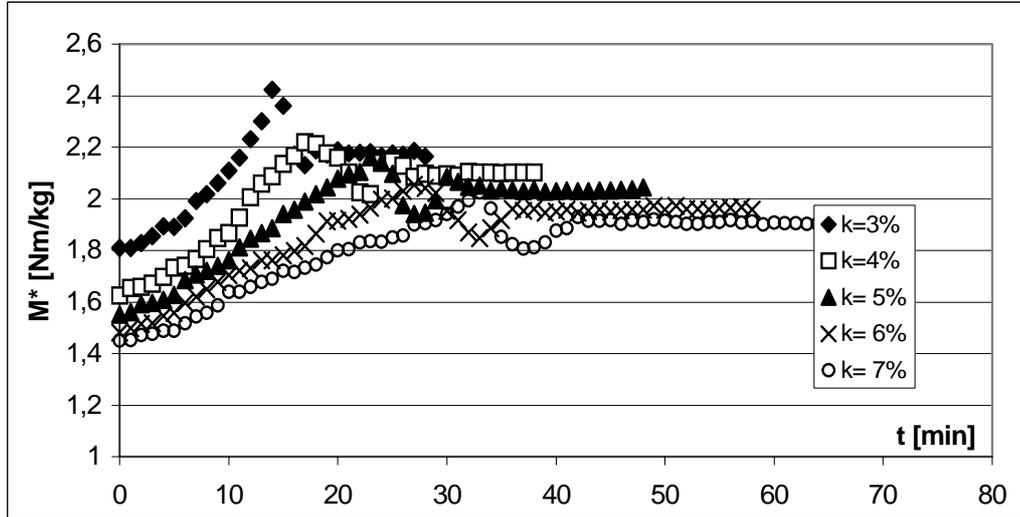
Fig. 3. Example of changes in reduced torque as a function of time for different values of disk filling  $k$  ( $D=1$  m;  $\alpha=47$ )
