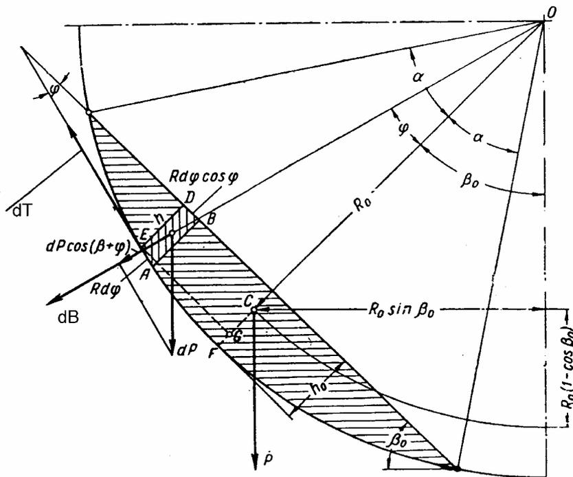
Fig. 1. Forces acting upon the elementary sector of the granulated bed
