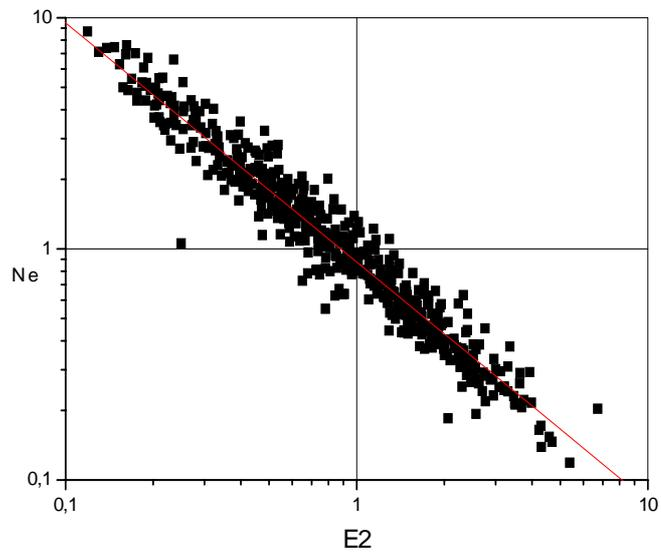
Fig. 4. Dependences of the power number on the value of  $E_2$  describing the effect of Froude number on process dynamics for the increase range
