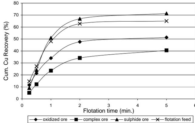
Fig. 5. Flotation behavior of the different ore types
