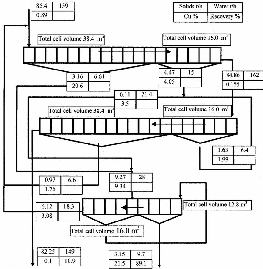
Fig. 2. Balanced flow rates, grades around the flotation circuit at actual operating condition
