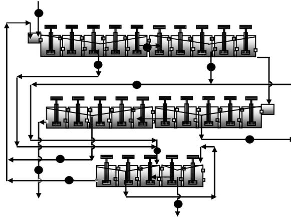
Fig. 1. Flotation circuits sampling points
