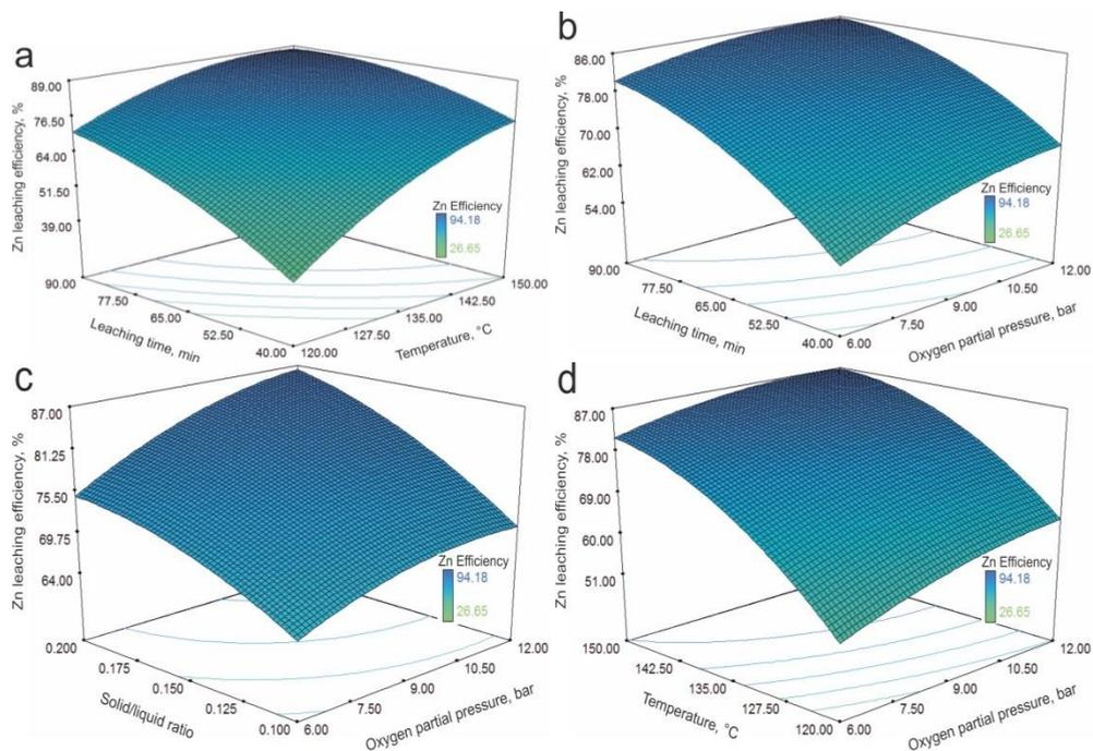
Fig. 5. Response surface plots showing the simultaneous effects of dual parameters on Zn leaching efficiency (other parameters are held at center level), (a) temperature and leaching time, (b)  $P_{O_2}$  and leaching time, (c)  $P_{O_2}$  and solid/liquid ratio, (d)  $P_{O_2}$  and temperature
