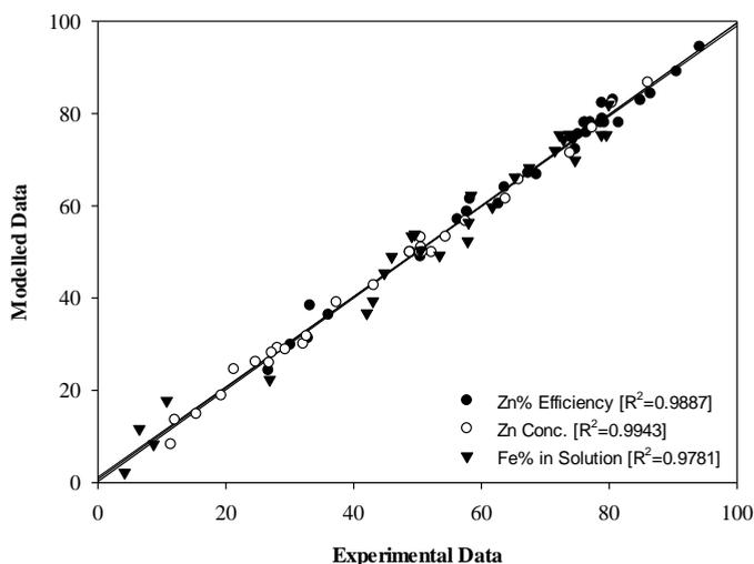
Fig. 2. Experimental vs. modeled data of all responses
