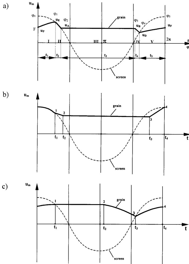
Fig. 1. Dependence of particle and sieve velocity on time
