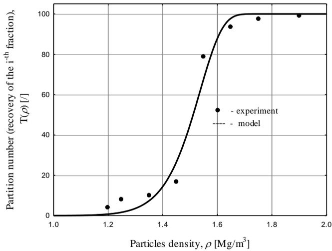
Fig. 5. Partition curve for 8–10 mm particle size fraction
