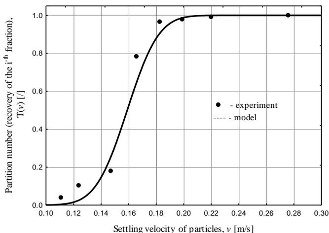
Fig. 4. Partition curve for tailing (8–10 mm size fraction)
