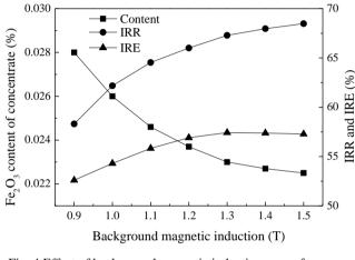
Fig. 4 Effect of background magnetic induction on performance. Conditions: rod matrix = 1.5 mm diameter wire and pulsating frequency = 50 rpm
