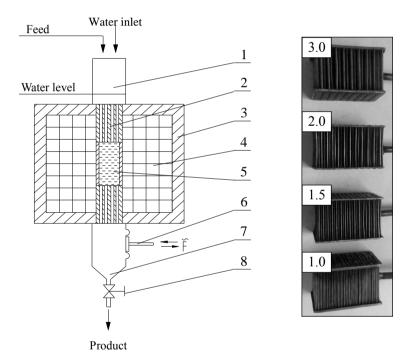
Fig. 1. Lab-scale PHGMS separator (left) and rod matrix of different wire diameters (right):
