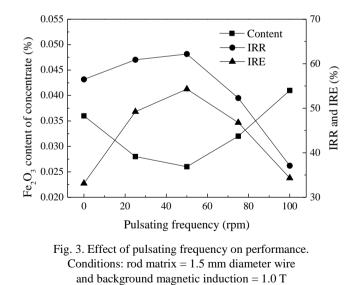
When the pulsating stroke was constant, the higher is the pulsating frequency, the more adequate is the pulsating energy in the separating zone of PHGMS separator (Xiong et al., 1998). From Fig. 3, the purification performance is not effective when
