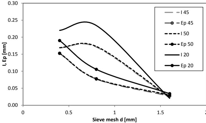
Fig. 2. Dependences of imperfection ( $I$ ) and probable error ( $E_p$ ) for the angles of 20, 45 and 50° for the sieves of 0.4, 0.8 and 1.6 mm (curves  $I_{50}$  and  $I_{45}$ , similarly as  $E_{p50}$  and  $E_{p45}$ , overlap)
