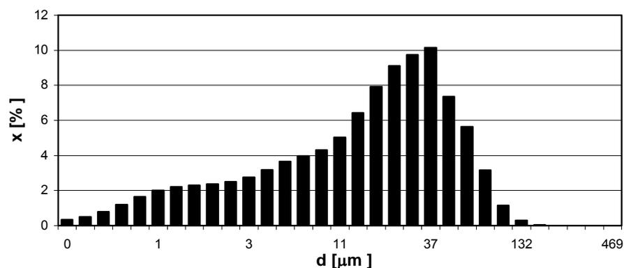
Fig. 1. Particle size distribution of silica flour MK 0.075
