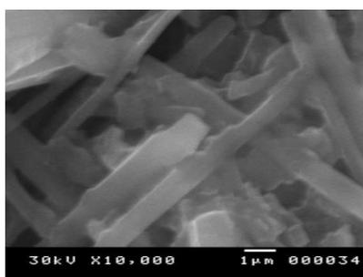
Fig. 4. SEM of gypsum crystals with 1 kg/Mg  $P_2O_5$  of sodium dodecyl sulfate
