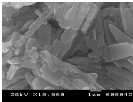
Fig. 3. SEM of gypsum crystals with 0.8 kg/Mg P<sub>2</sub>O<sub>5</sub> of sulfonic acid
