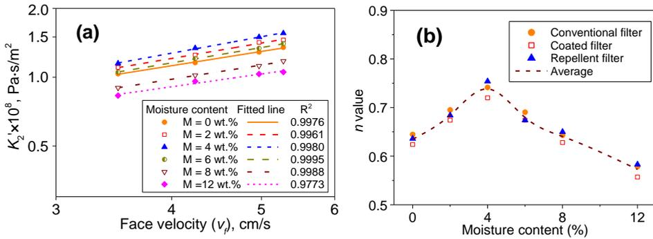
Fig. 6. Correlation curves of (a) the specific resistance  $k_2'$  as a function of the face velocity, and (b) the compression coefficient  $n$ , which was obtained from the relationship between  $k_2'$  and  $v_f$ , as a function of moisture content
