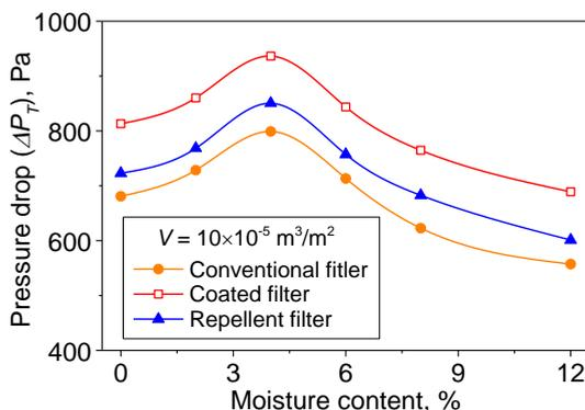
Fig. 4. Filtration pressure drop as a function of the moisture content when a loaded dust true volume  $V = 10 \times 10^{-5} \text{ m}^3/\text{m}^2$  was utilized for the conventional, coated, and repellent filters
