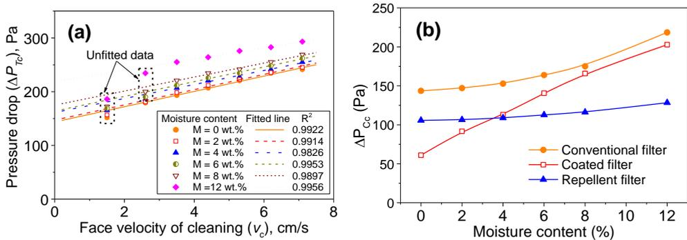
Fig. 10. Pressure drop upon cleaning where the filtration face velocity  $v_f = 4.24$  cm/s: (a) total pressure drop as a function of the cleaning face velocity, obtained using conventional filter, and (b) pressure drop in the cake as a function of the moisture content for the conventional, coated, and repellent filters
